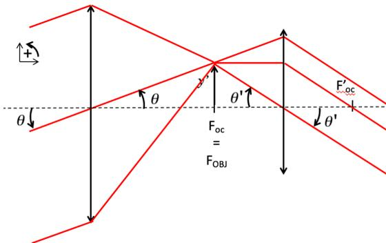
2.  $d_{\text{obj-oc}} = f'_{\text{obj}} + f'_{\text{oc}} = 880\text{mm}$
