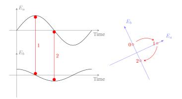
**Figure 4.4** – Illustration of the relation between phase shift sign and sense of rotation of the ellipse.
