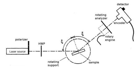
Figure 3.2 - Set-up scheme
