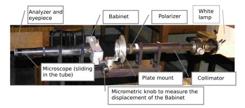
Figure 2.3 – Experimental setup
