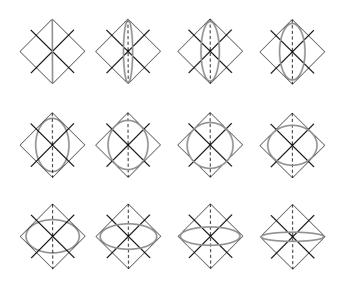
Figure 4.7 – Resulting ellipses with respect to the dephasing introduced by the birefringent plate. The incident polarisation is represented by a bold grey line when the phase is null and dashed otherwise. Its orientation stands at 45° from the neutral axes of the plate appearing in bold black lines.
