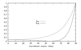
Figure 3.1 – Intensity coefficient of reflection  $R_{TE}$  and  $R_{TM}$  versus the incidence angle (standard glass n = 1,515 at 633 nm)
