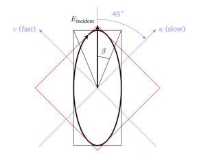
Figure 4.6 – Ellipse at the output of a nondescript birefringent plate.
