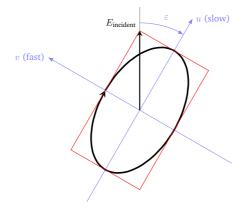
**Figure 4.5** – Ellipse at the output of a quarter wave plate for a linear input polarisation. The ellipticity is indeed the angle between the direction of the input polarisation and the neutral axis of the QWP.
