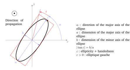
Figure 4.3 – Elliptic polarisation properties
