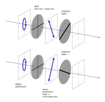
**Figure 4.8** – Illustration for the quarter "waveplate method" to measure the ellipse's main parameters.
