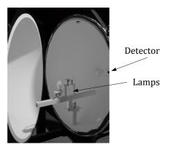
Figure 2.1 – The integrating sphere from LabSphere at LEnsE.
