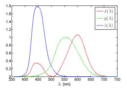
**Figure 4.1** – Definition of the XYZ tristimuli starting from the spectric energetic luminance
