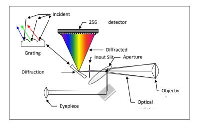
Figure 1.2 - Principle of a PhotoResearch spectroluminancemeter.
