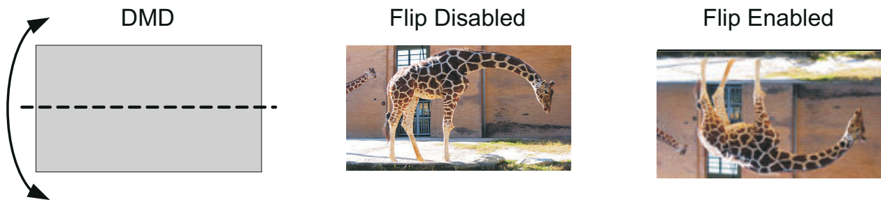
Figure 2-2. Image Short-Axis Flip Example
