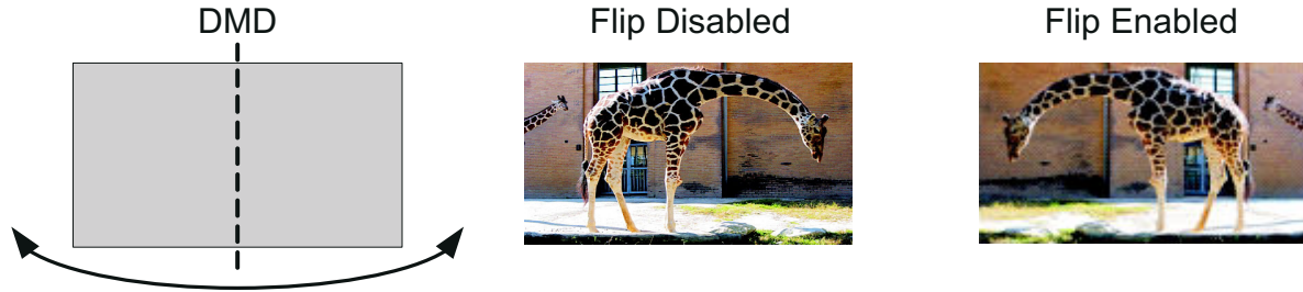
Figure 2-1. Image Long-Axis Flip Example
