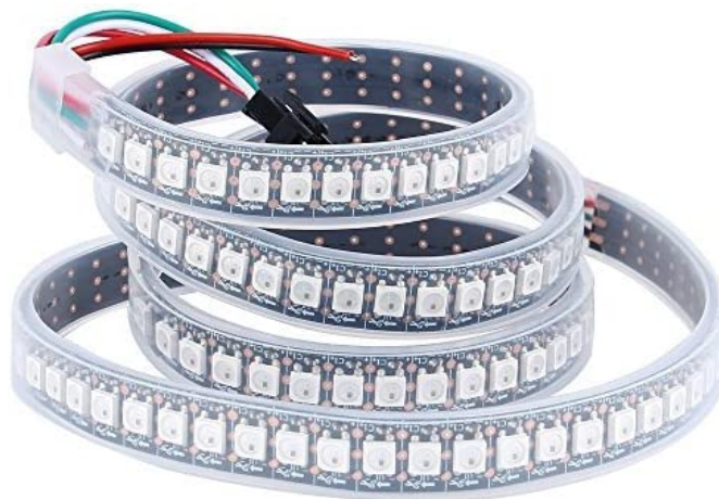
Figure 5: Bande de Led WS2812b
