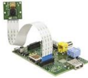
Figure 3 - Raspberry Pi et appareil photo ( http://liyao.me/raspberry-pi-wifi-camera/ )
