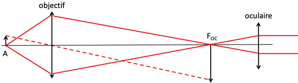
2.  $g_{y-obj} = -3 = -\frac{\overline{F'A'}}{f'_{\text{objectif}}} = \frac{f'_{\text{objectif}}}{\overline{FA}} \longrightarrow \begin{cases} \overline{OA'} = 160\text{mm} \\ \overline{OA} = -53,3\text{mm} \end{cases}$
