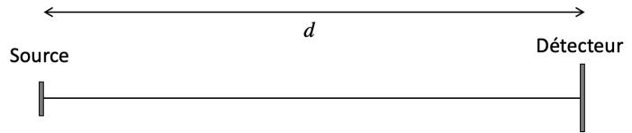
$$F_D = L_s \times G_{source-déTECTeur} \approx L_s \times \frac{S_s \times S_D}{d^2} = 2,5 \text{ pW}$$
