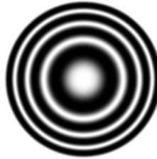
Figure 3.6: Out of focus in relation to the paraxial focus (FOCUS = 2\lambda )
