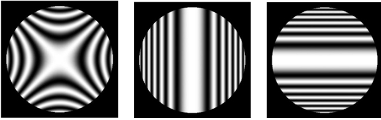
Figure 3.9: Astigmatism (ASTIGMATISM = 3\lambda ). Left: Spherical mirror at the best focus
