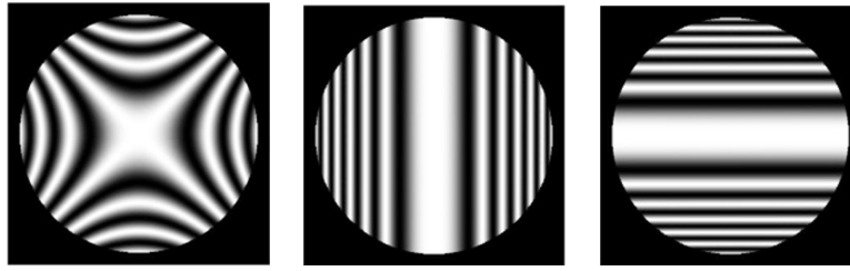
Figure 3.9 – Astigmatism ( \text{ASTIGMATISM} = 3\lambda ). Left: Spherical mirror at the best focus
