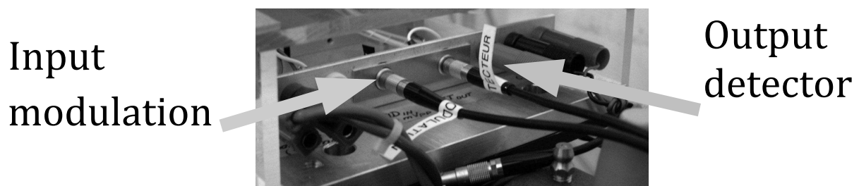
Figure 2.3 – Connectors used for the detector output and the modulation input.
