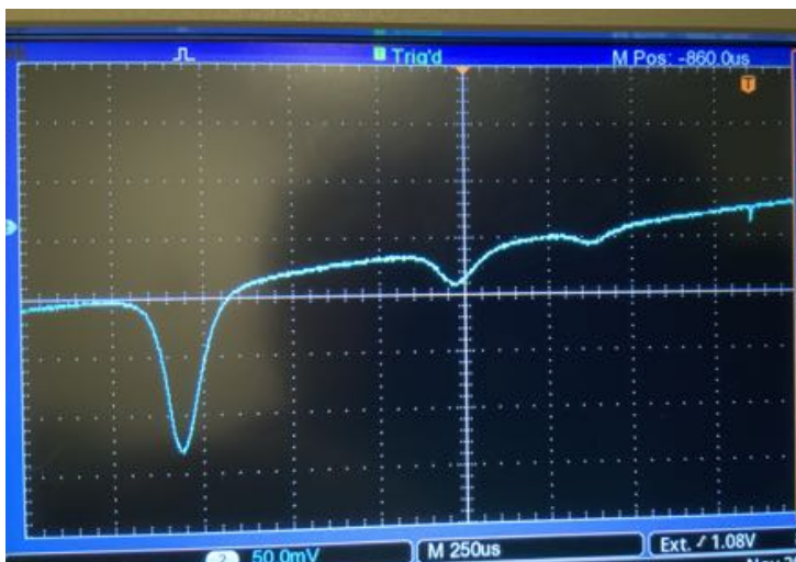
Figure 5.4: Absorption spectrum through the atomic jet. This spectrum was obtained using the same set-up as the one you have, by measuring the laser intensity transmitted through the vacuum chamber and the atomic jet, using an amplified photodiode and sweeping the frequency of the laser diode.
