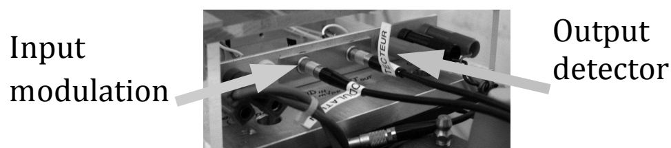
Figure 2.3 – Connectors used for the detector output and the modulation input.
